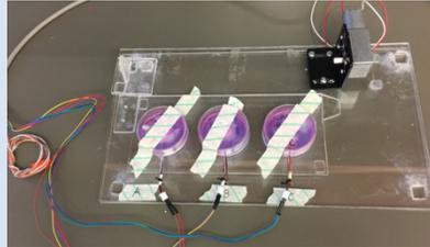
**Fig 1.** Bioreactor with transducers and signal generators
