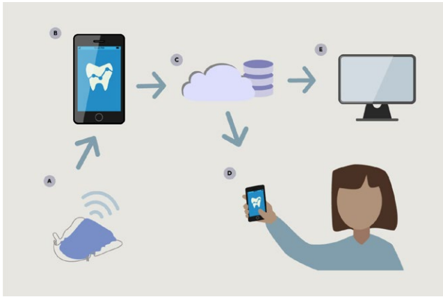
FIGURE 2 Overview of the Retainer System. A, Bluetooth-enabled retainer; B, Patient's mobile phone or iPod touch; C, Wear time data stored to the cloud; D, Patient receives real-time feedback, rewards, etc.; E, Secure provider webpage
