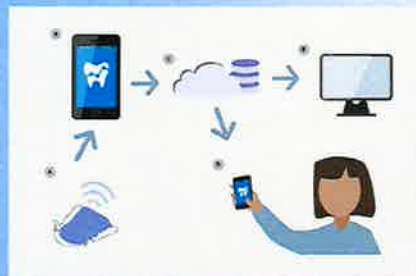
Figure 2: Overview of the Innov8 System. (A) Innov8 Retainer; (B) Patient's mobile phone or iPod touch; (C) Wear time data stored to the cloud; (D) Patient receives real-time feedback, rewards, etc; (E) Secure provider webpage
