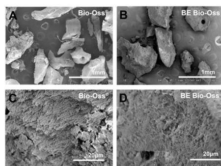
Figure 2. Electron microscopic comparison of Control Bio-Oss<sup>®</sup> and BE Bio-Oss surface structure. (A,B) are SEM at 45-fold magnification, (C, D) and 1500-fold magnification. (A, C) are from commercial grade Bio-Oss<sup>®</sup> as control, and (B, D) are from BE Bio-Oss. A scale bar in the right serves as a references for the level of magnification.
